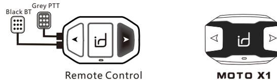
First of all, unplug all the cables on the **MOTO X1** and switch it off. Press and hold [▶] and grey PTT button on the remote control, then press [id] to switch on the main unit to let both remote control and main unit enter into pairing mode. When the pairing is completed, the indicator on the **MOTO X1** will blink green for 3 seconds. After the pairing is finished, buttons on remote control will have the same functions as the buttons on the main unit.
