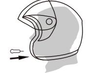
Refer to the user's mouth position, install the microphones onto the cushion of both sides.
