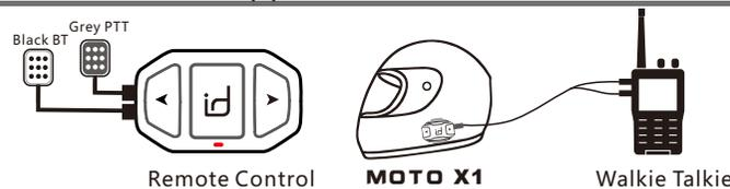
After pairing the remote control with **MOTO X1**, press and hold the PTT button on the remote control can control the PTT function of the walkie talkie.
