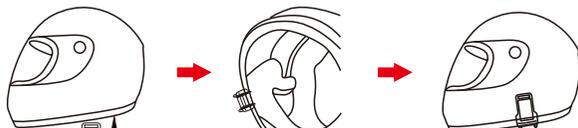
Position and fasten the clip bracket onto the helmet.
