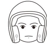
The two microphones and user's mouth must be on the same horizontal level.
