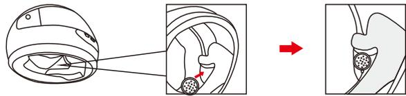
Use the Velcro to install the speakers into the ear cavity of the helmet.
